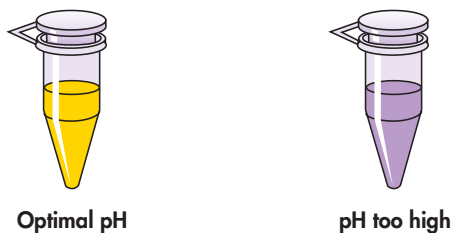
Figure 3 Indicator dye in solubilization and binding Buffers QG and ERC identifies optimal pH for DNA binding.
