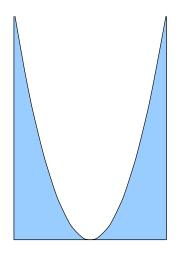
The ideal refracting lens has a parabolic shape but this is impractical to make.
